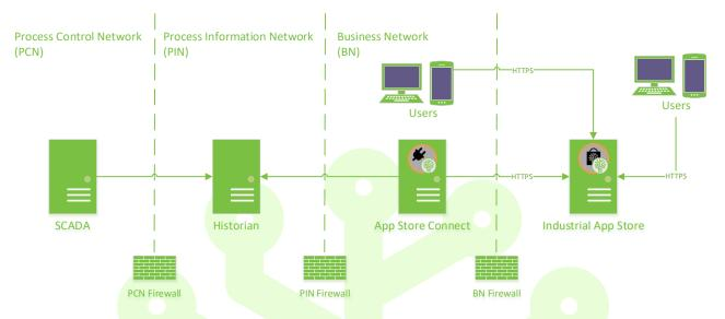
The above diagram illustrates a typical architecture - directions of arrows indicate the direction in which a connection is initiated. App Store Users (internal and external) can only access business data from the Industrial App Store through the secure App Store Connection.
